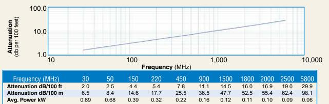
Calculate Attenuation = (0.356859) • FMHz + (0.000470) • FMHz (interactive calculator available at http://www.timesmicrowave.com/cable\_calculators)
